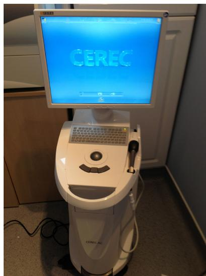
There are two parts to this: a computer on the trolley with a little camera on it and then the milling machine. If you were going to have a crown or a filling, instead of taking a mould like you normally do, you scan the tooth with the camera into the computer, design the restoration and then beam that to your milling machine. You can mill your own restoration in about 15 minutes.
