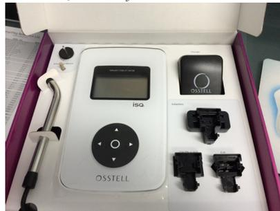
When you place a dental implant you normally wait three months to place the crown, but the implant hasn't always integrated into the jaw bone. This machine will tell you when it has.
